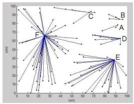
Fig. 2. Cluster head formed in Leach protocol [6]
